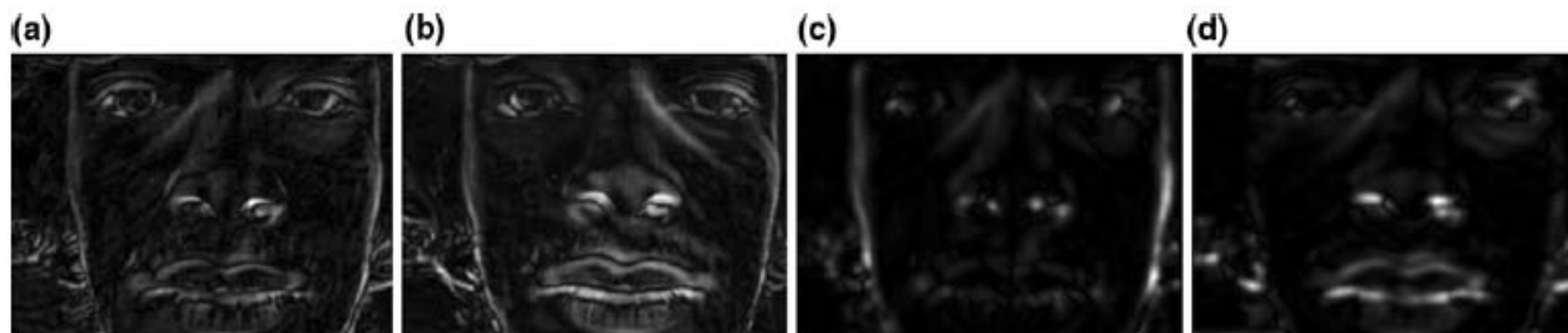
Fig. 5 a High-pass flicker (Flicker); b low-pass flicker (Flicker-N); c horizontal optical flow ( U -Flow); d vertical optical flow ( V -Flow) for the frame in Fig. 1a
